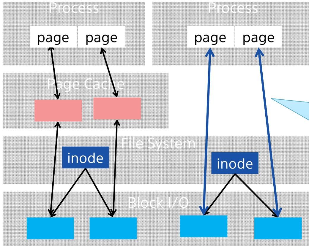
Data in userland will be stored directly to the storage device without CPU workload.
