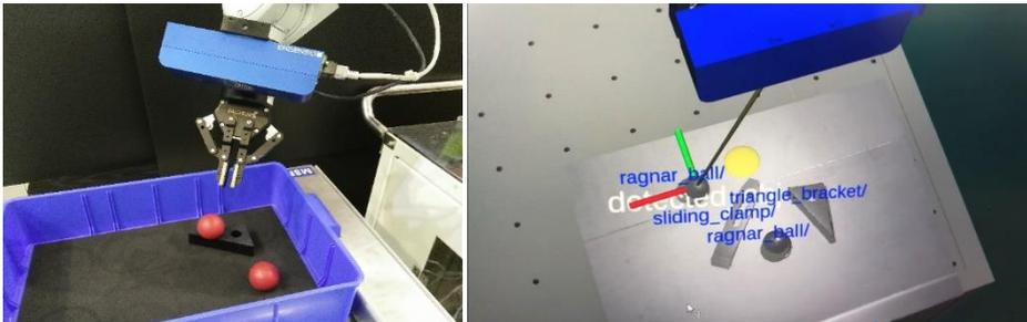
ROS allows for real time visualization of sensor data
