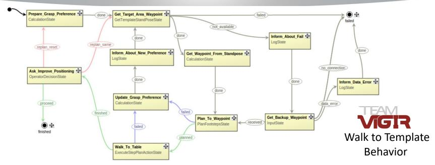
A state machine realizes a desired "behavior" by invoking system capabilities;
