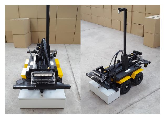
Fitted with; 2x 20m (Hokuyo) LIDARS for full 360°FOV, 2x 3D point cloud (Orbbec) RGB camera, 1x Top down HD Web camera, 2x Super bright LED Spot Lights and 1x Ring of RGB LEDs for signalling Operators
