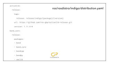
The rosinstall\_generator tools uses as its source data the distribution.yaml which governs which version of every package is the current latest in a given distribution. So in this case, version 1.11.6-0 was the last bloomed release of actionlib into ROS Indigo. The build farm uses this data to generate Jenkins jobs to build debian packages, but rosinstall\_generator uses it to generate source workspaces.
