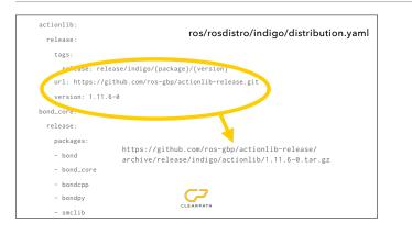
The generator is capable of generating a list of git URLs, but downloading tarballs is much faster than cloning git repos, so there is logic to recognize known git hosts and supply tarball URLs with the --tar flag.
