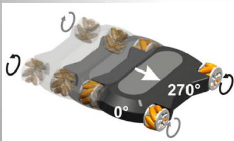
moving sideways wheels rotate in opposite directions
