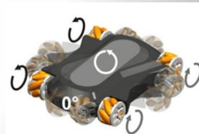
rotate around central axis wheels on one side rotate in opposite direction to wheels on other side
