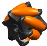
Meccanum wheel with passive rollers
